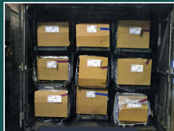
This truck is completely loaded with Astro racks, eliminating bundle-to-bundle contact and hence, damage.
